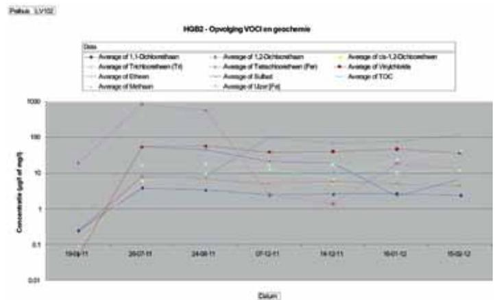
Decreasing 1,2-dichloroethane levels in the monitoring well prove biodegradation in the HGBcell
